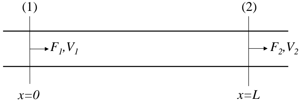
Figure 2. Relationship between amplitudes of force and velocity at different stations along elastic rod.
